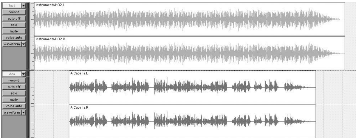
FIGURE 7.3 The Instrumental and A Cappella . An a cappella version of a song lined up with its radio version in Pro Tools . Since the vocals of the a cappella version line up with the vocals of the radio version, we know that their tempos are identical and that it's okay to figure out the song's tempo using a loop from the radio version.
